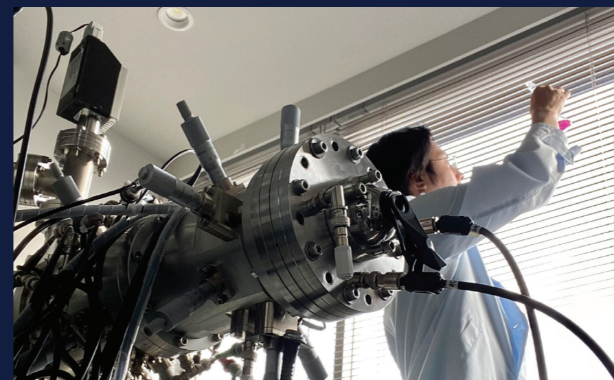
Developing the mass separator, which generates elementally selected ion beams
