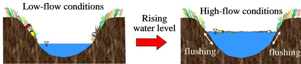
**Figure 1** Fundamental mechanism for flushing of vegetation and debris as sources of floating litter in rivers.
