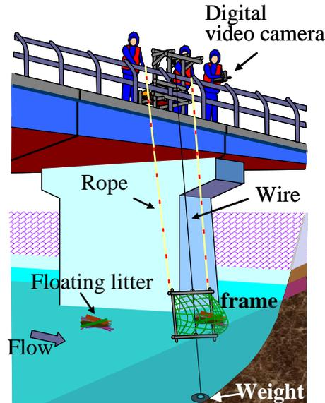
**Figure 3** Schematic view of direct collection of floating litter.
