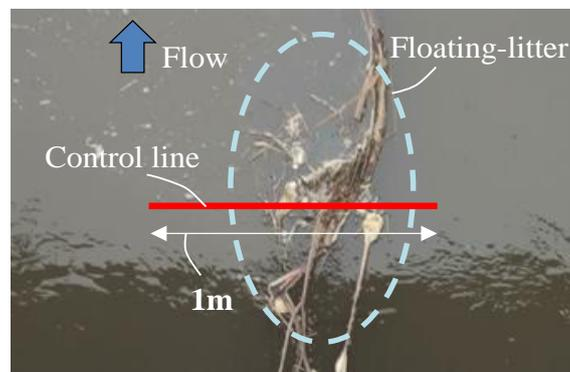
**Figure 4** Example of image of floating litter in video monitoring.
