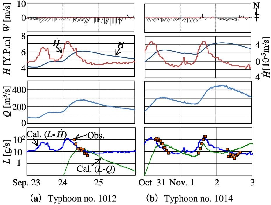
**Figure 5** Temporal variations of wind velocity vector  $W$ , water elevation  $H$ , temporal variation rate in water elevation  $\dot{H}$ , discharge  $Q$ , and floating litter transport  $L$ .
