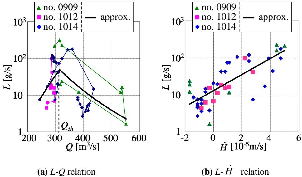
**Figure 6** Rating curves for floating litter transport.
