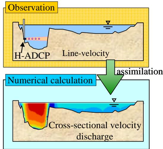
**Figure 1.** Fundamental structure of present monitoring system
