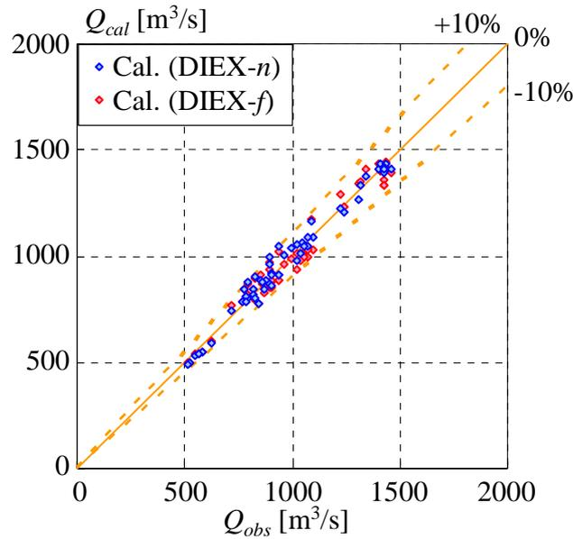
**Figure 6.** Comparison of the observed discharge  $Q_{obs}$  and calculated discharge  $Q_{cal}$  in events 1 and 2 for all.
