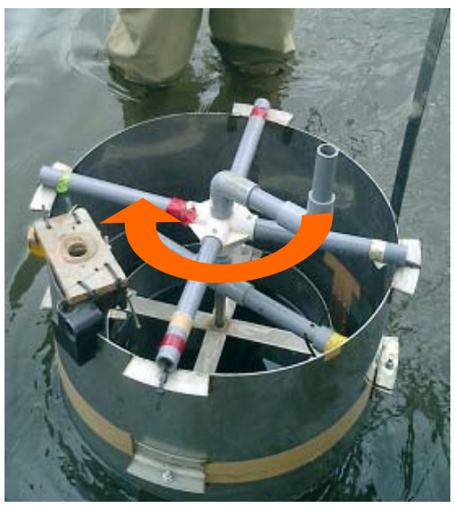
Figure 1. Schematic diagram (upper) and photographs (lower) of our new device for in-situ measuring of pick-up rates of sediment and nutrients
