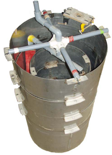
Figure 1. Schematic diagram (upper) and photographs (lower) of our new device for in-situ measuring of pick-up rates of sediment and nutrients
