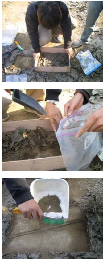
Figure 4. Actual procedure for collecting sediment deposited in a reservoir.
