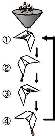
Fig. 2 Conceptual view of the measurement of deposition sediment flux using the tipping bucket.
