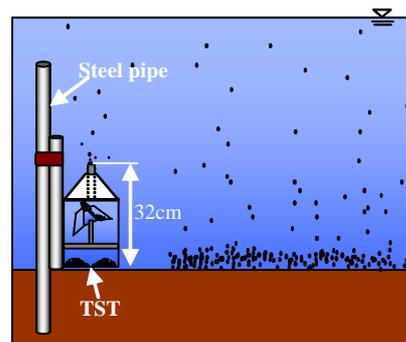
Fig. 7 Schematic view of the TST mounted in the rivers.
