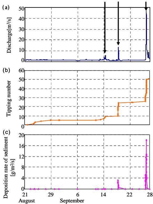
Fig. 8 Temporal variations in river discharge (a); tipping number (b); and, deposition rate of sediments (c) in the Oohori River.
