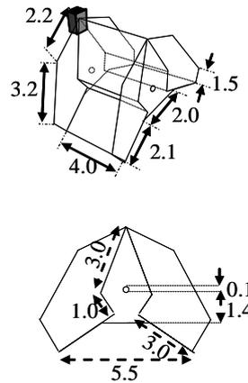
Fig. 3 Configuration and dimensions of the tipping bucket. (Unit:cm)
