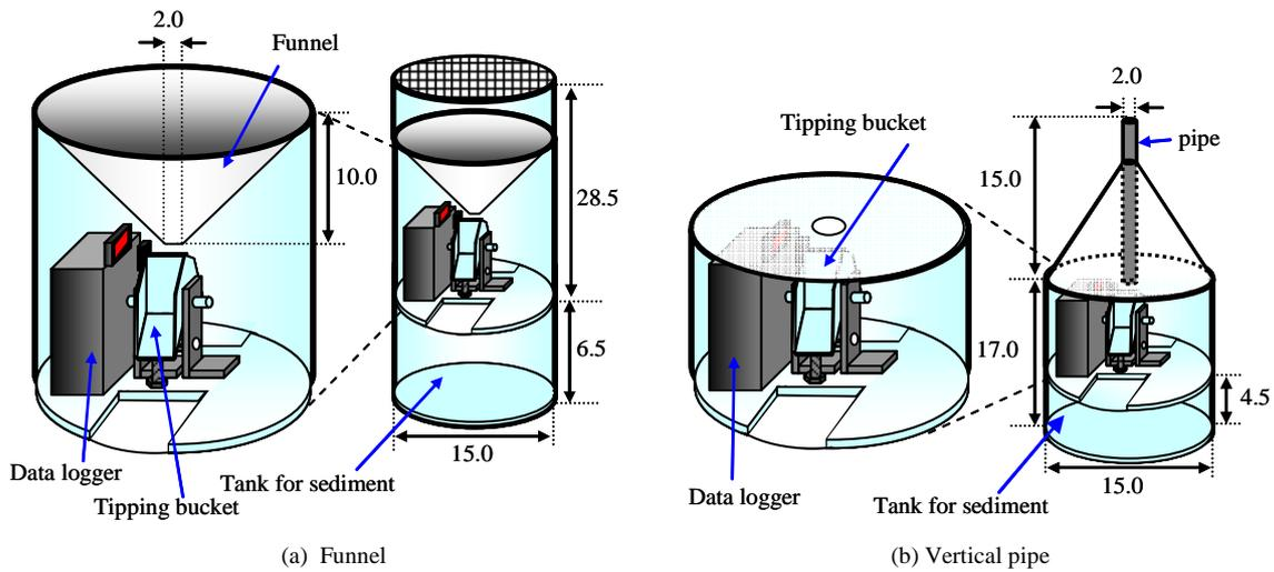
Fig. 1 Schematic view of the tipping-bucket sediment trap fitted with funnel and vertical pipe collection devices.(Unit:cm)
