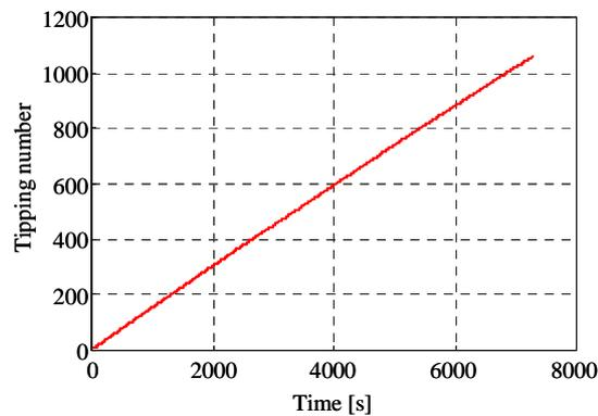
Fig. 5 Temporal variation of the tipping number using the TST fitted with the vertical pipe.
