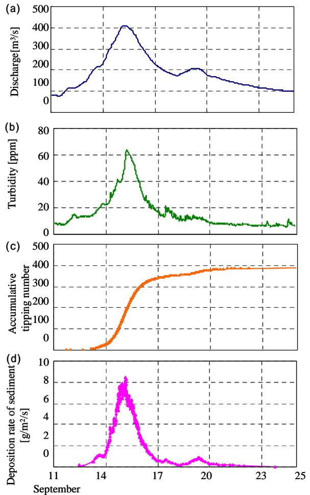
Fig. 9 Temporal variations in river discharge (a); turbidity (b); tipping number (c); and, deposition rate of sediments (d) in the Edo River.
