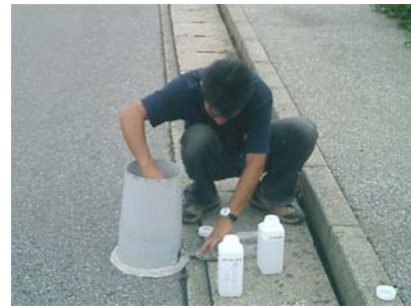
Fig. 3 Photograph for the measurement of road-deposit environments with the MOS technique.
